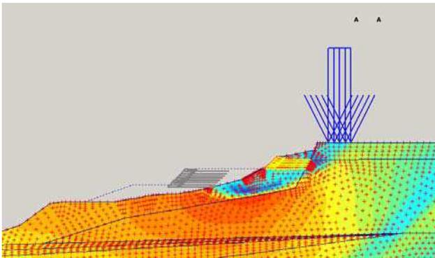
Figure 6. Simulated state of failure for the execution of the first retaining wall only
