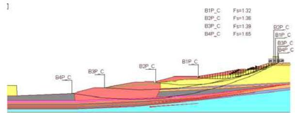
Figure 7. Analysis of stability for profile B-B
