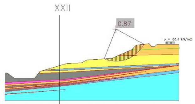
Figure 1. Analysis of stability for profile IV according to the condition on the 8 November 2002
