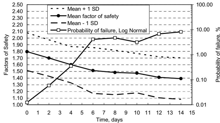
Figure 5. Factor of safety and probability of failure with time
