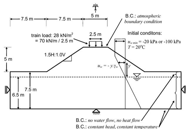
Figure 3. Embankment geometry, initial, and boundary conditions
