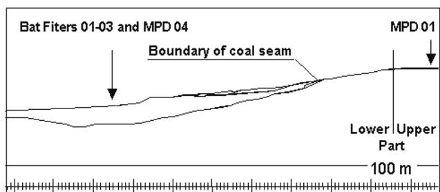
Figure 5. Typical section through unstable part of the open cast mine
