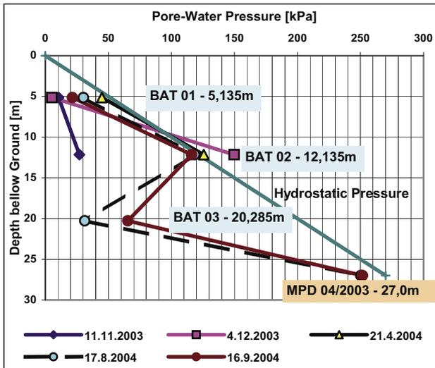
Figure 6. Example of pore-water pressure monitoring in spoil heap
