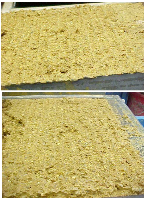
Fig.8. Typical shear surface of the soil-cement grout interface shear tests under a lower applied normal stress 50kPa in the natural wet condition – (a) cement grout failure surface (top), and (b) soil failure surface (bottom) (after Chu and Yin 2005)
