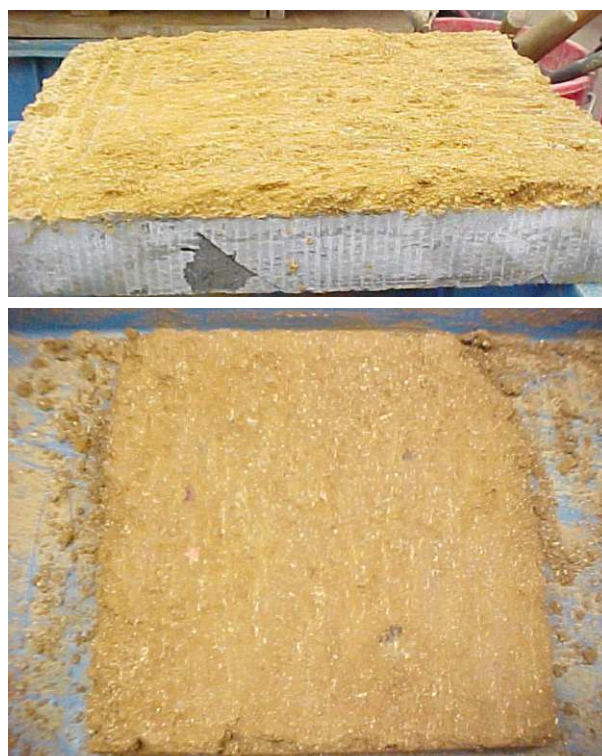
Fig.9. Typical shear surface of the soil-cement grout interface shear tests under a higher applied normal stress 300kPa in the natural wet condition – (a) cement grout failure surface (top), and (b) soil failure surface (bottom) (after Chu and Yin 2005)
