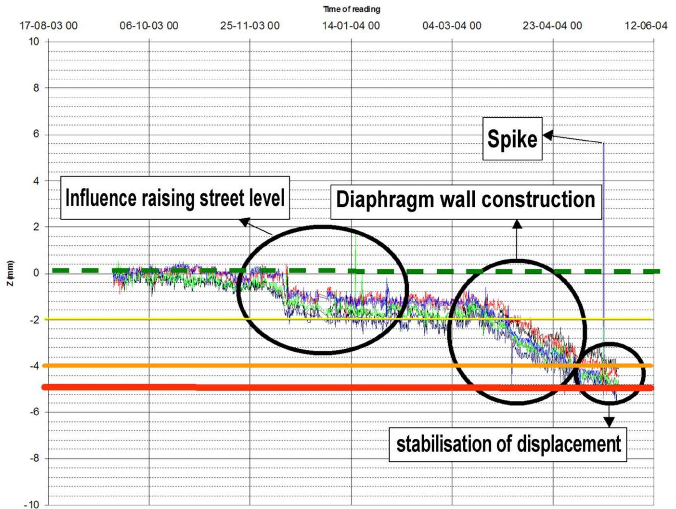
figure 3: Example of displacement lines around Ceintuurbaan station
