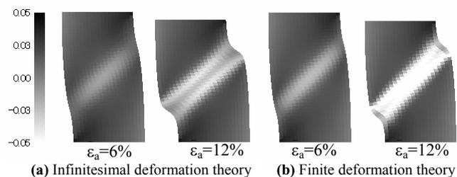
Figure 4 Distribution of volumetric strain for 2D (OCR=10)
