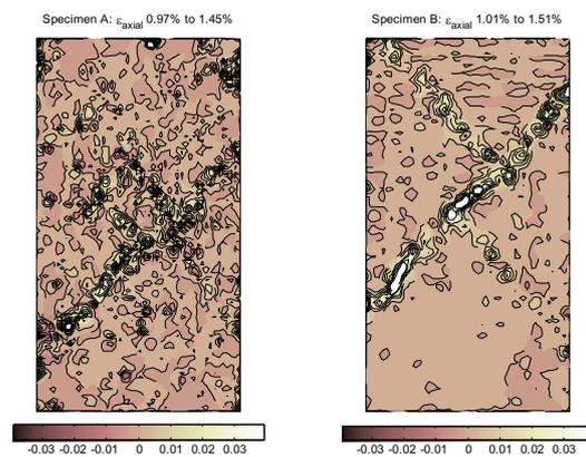
Figure 5. Contours of the incremental volumetric strain levels for dense two-dimensional specimens close to the point at which the peak stress is mobilized: Specimen A contains 5,728 disks (left) and Specimen B has 12,532 disks (right) (*O'Sullivan and Bray*)
