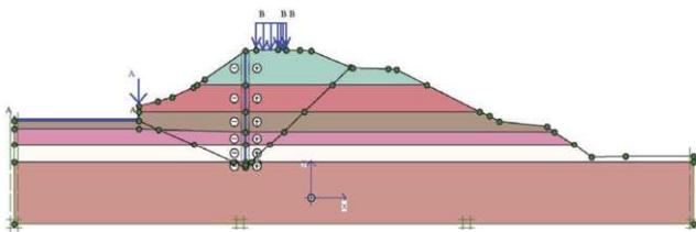
Fig.2 River dike strengthened with sheet pile
