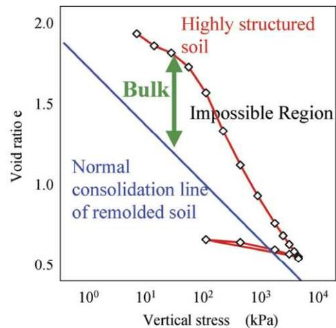
Fig.3 Compression curve of structured soil
