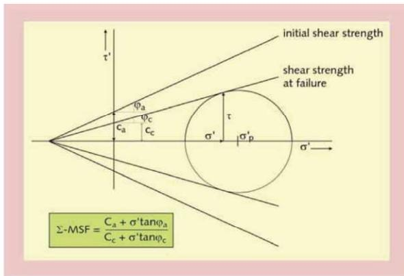
Fig.1 Phi-C reduction method
