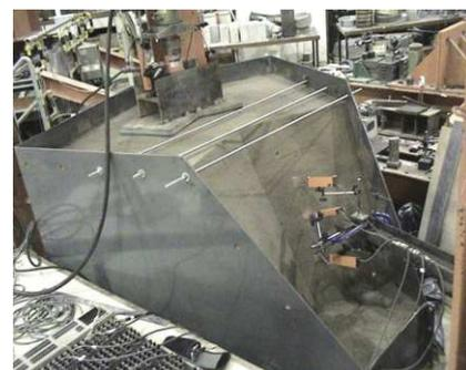
Photo 1. Model experiments for soil nails in The Hong Kong Polytechnic University
