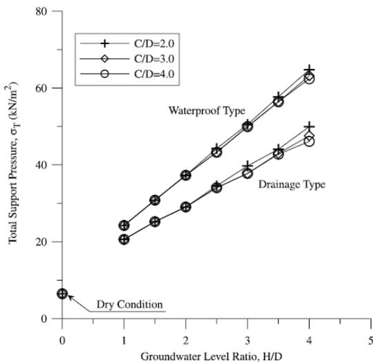
Figure 1. Change of support pressure with variation of the  $H/D$  ratio
