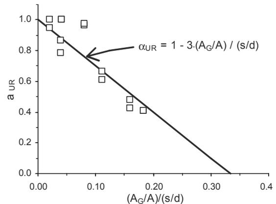
Figure 1. Relationship between  $\alpha_{UR}$  and filling factor  $FF = (A_G/A_R)/(s/d)$
