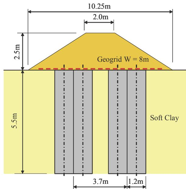
Figure 29. RF combined with deep mixing.
