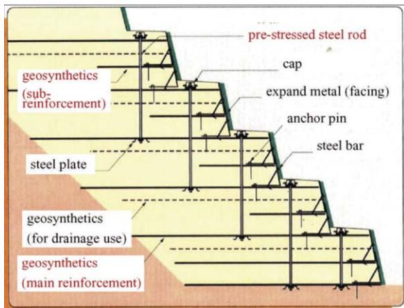
Figure 23. RE combined with drainage, preloading and prestressing.
