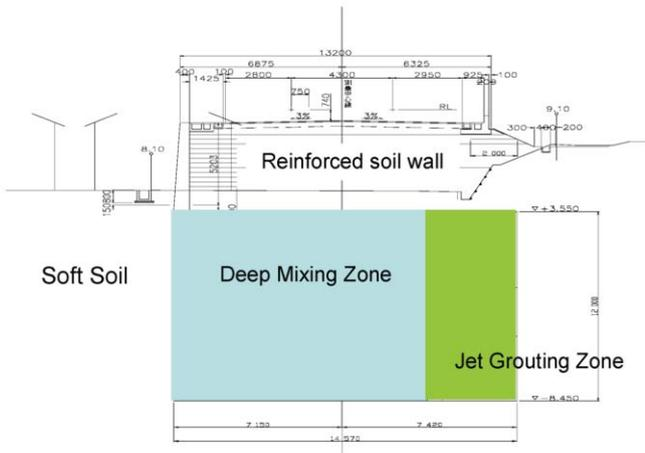
Figure 19. RSW with deep mixing and grouting.
