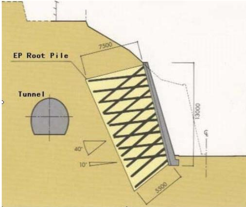
(b) Reinforcing soil for cutting slope
