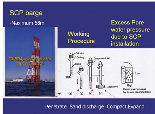
Figure 12. Sand Compaction Pile Method (from presentation by Dr. Nozu)
