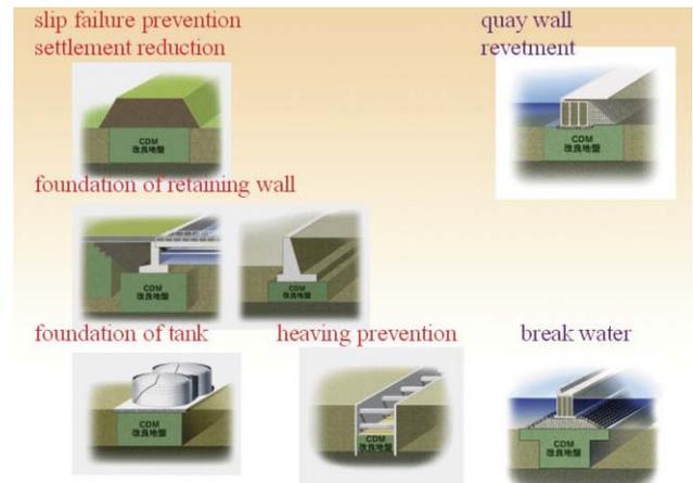
Figure 11. Development of Pneumatic Flow Mixing Method and its Application (from presentation by Dr. Kitazume)
