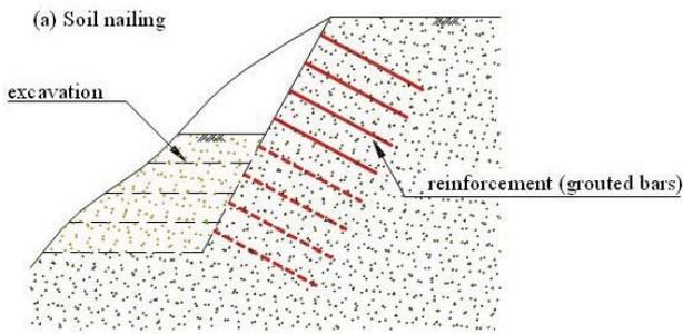
(a) Reinforcing soil for excavation technique
