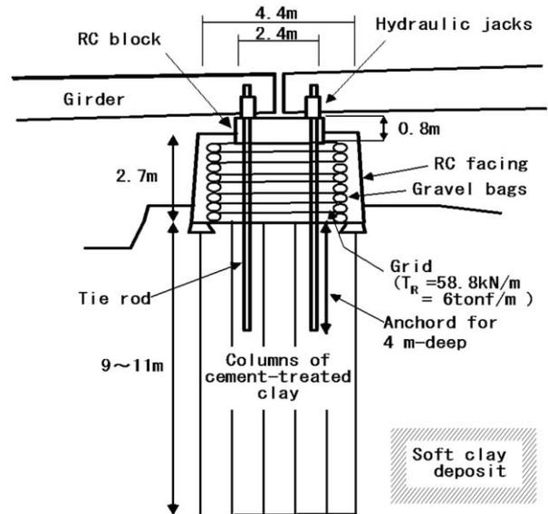
Figure 21. RSW combined with preloading and prestressing.
