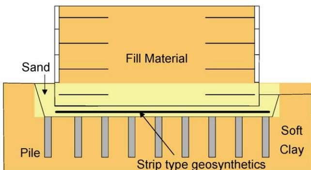
Figure 28. RF combined with piles
