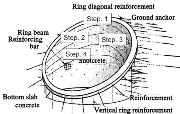
Figure 27. Nailing combined with ring reinforcement.
