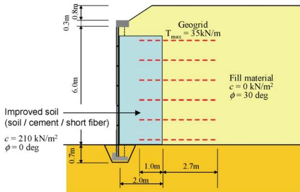
Figure 17. RSW combined with mixing of cement and short fiber. (From Dr.Hirai, member of Japanese Supporting Committee)
