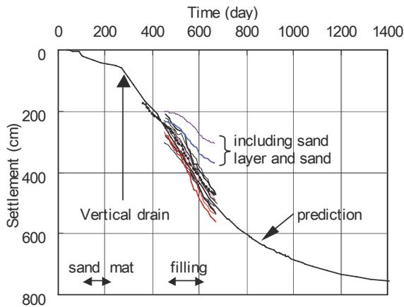
Figure 10. Evaluation of design of ground improvement by monitoring results (from presentation by Dr. Katagiri)
