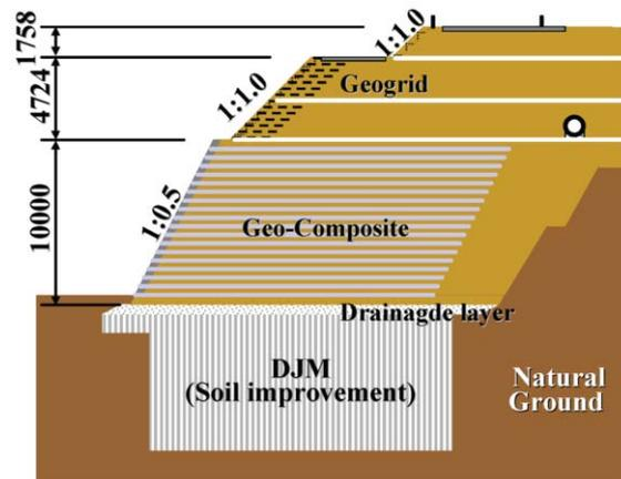
Figure 22. RE combed with drainage.
