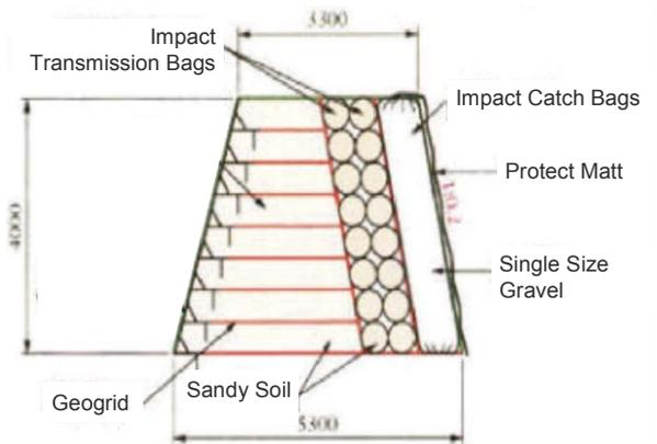
Figure 24. RE combined with impact absorber.
