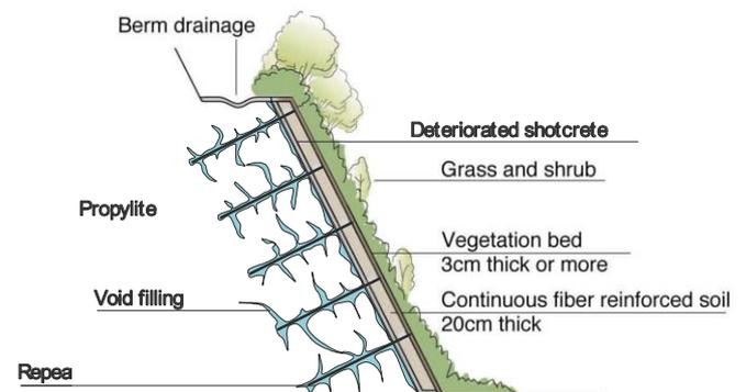
Figure 26. Nailing combined with fiber reinforced soil.
