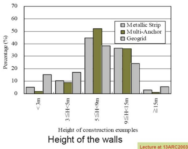
(b) Frequency of scale of constructed reinforced soil wall in Japan
