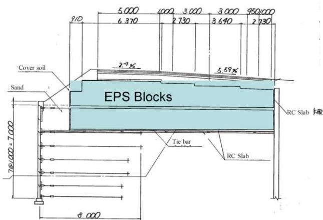
Figure 20. RSW combined with EPS Blocks.
