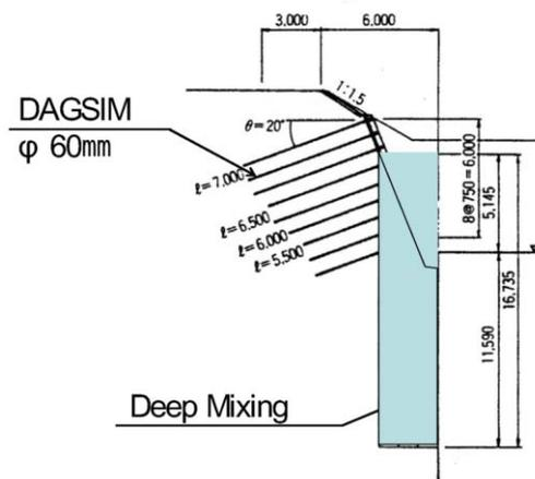
Figure 25. Nailing combined with deep mixing.
