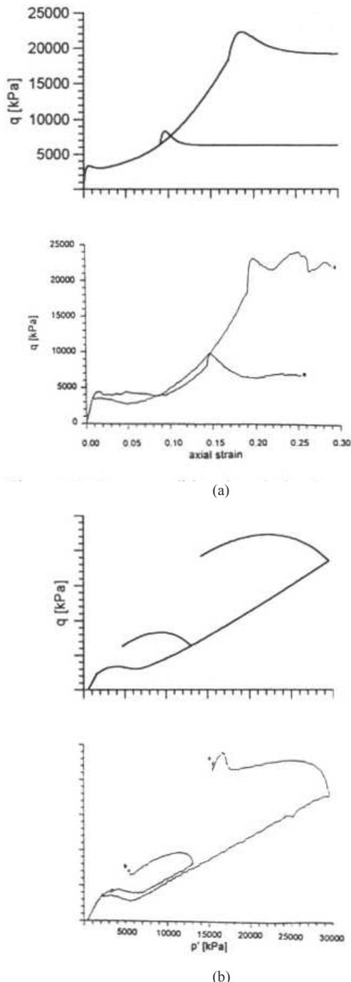
Figure 4. Undrained tests after  $K_0$  consolidation on Stevn's Klint chalk: calculated results (above) from Nova and Lagioia (1996) and experimental data from Leddra (1988). a) stress strain relationship b) stress path.
