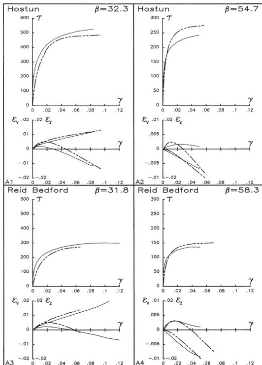
Figure 1. Comparison of experimental and predicted results in four drained hollow cylinder tests on sand: constant cell pressure and constant angle between major principal and vertical stress expressed in degrees (After Nova, 1988)
