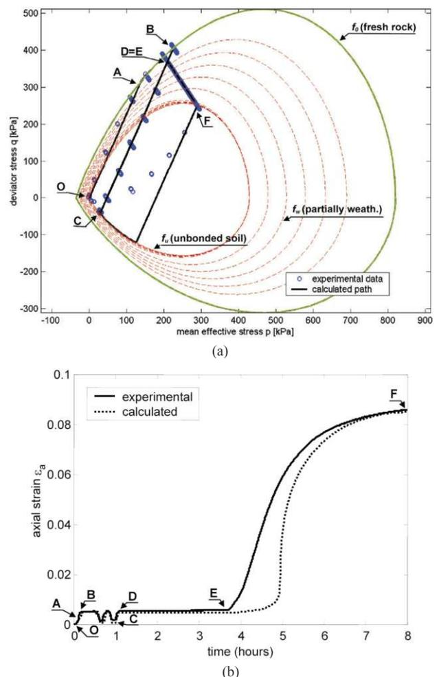
Figure 5. Lime cemented silica sand: oedometric loading followed by chemical attack at constant axial load and final unloading: a) stress path; b) variation of axial strain with time (after Nova et al., 2003).
