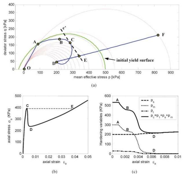
Figure 6. Predicted behaviour in a strain-controlled oedometric test on a bonded material: (a) stress path in the  $q$ - $p$  plane (Point  $C$  corresponds to the maximum value of axial stress  $\sigma_a$ ); (b) stress-strain response in the  $\sigma_a$ - $\epsilon_a$  plane; (c) evolution of internal variables (after Nova et al., 2003).
