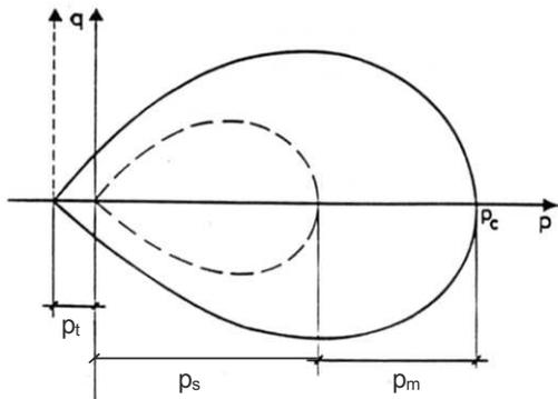
Figure 2. Modification of elastic domain due to cementation
