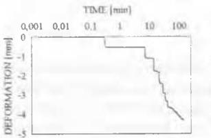
Figure 5. Laboratory settlement vs. time curve for angular grains.
