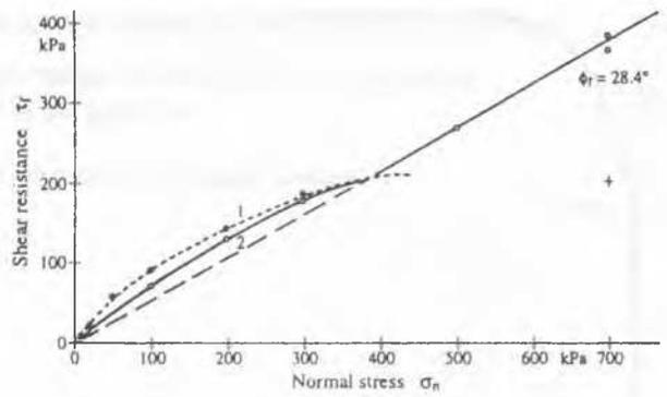
Figure 15. Effect of initial porosity on debonding surface of sand treated by 2% of cement. 1:  $n_0 = 50\%$ ; 2:  $n_0 = 55\%$ .
