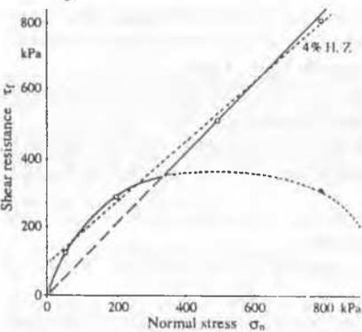
Figure 13 Shear strength and two interpretations of the strength envelope of dense saturated sand with 4% of cement.
