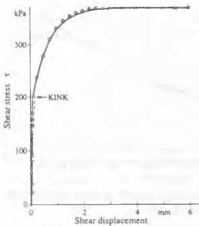
Figure 16. Identifying the point of debonding <+> of Figure 15.
