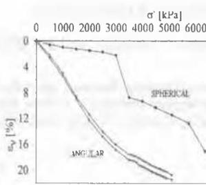
Figure 4. Compression of angular and spherical grains.
