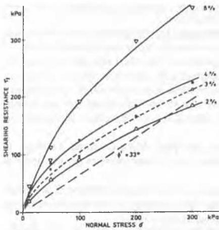
Figure 11. Non-linear shear strength envelopes for sand cemented by 2% to 8% of Portland cement (Feda, 1998).
