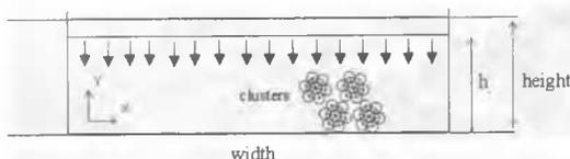
Figure 7. Scheme of the numerical oedometer test
