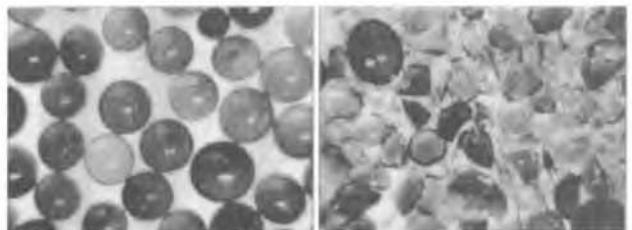
Figure 1. Silicagel 2-4 mm prior oedometer testing. Figure 2. Silicagel 2-4 mm after oedometer testing.
