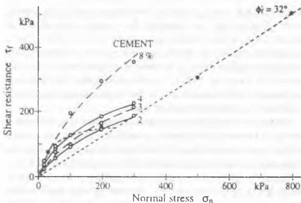
Figure 17. Effect of the amount of cement on debonding surface.
