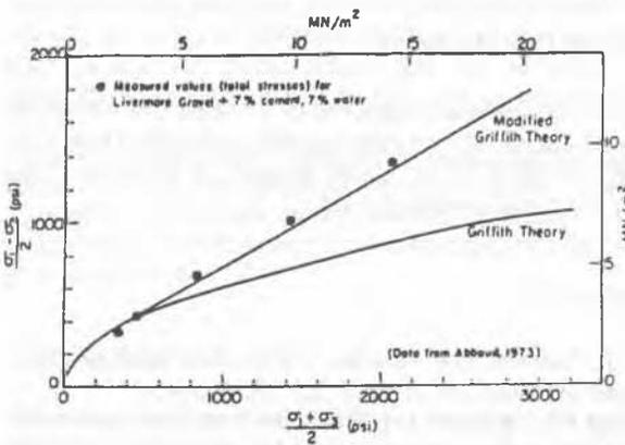
Figure 12. Strength envelopes of cement-treated gravel: experiments and Griffith theory (Mitchell, 1976).
