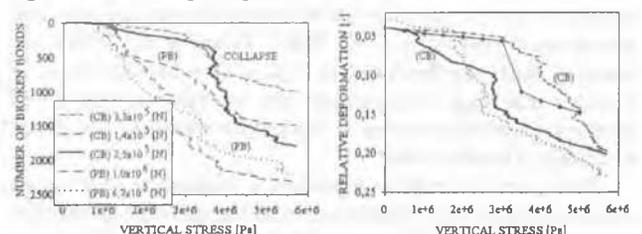
Figure 9. Numerical compression curves.
