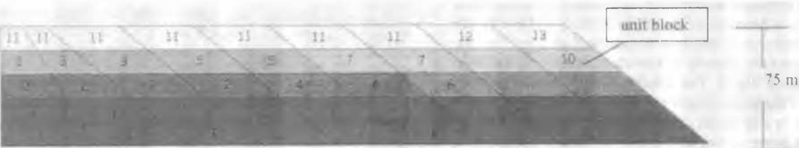
Figure 6. Banking up a salt stockpile in blocks
