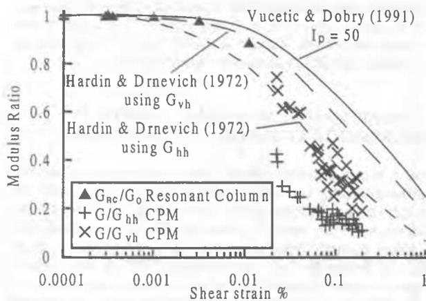
Figure 6: Resonant column data from the Madingley site
