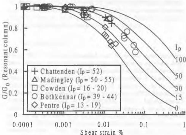
Figure 4: Resonant column data with Vucetic & Dobry (1991) curves
