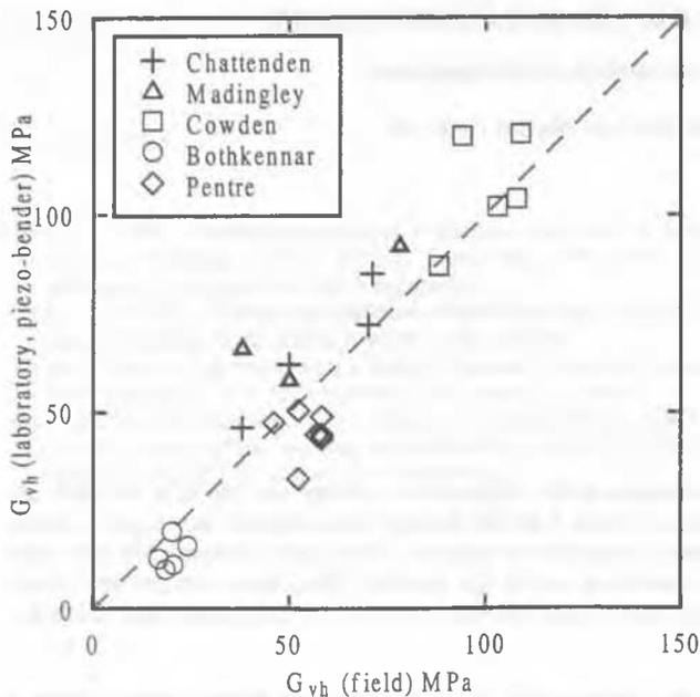
Figure 1: Comparison of stiffness derived from field and laboratory shear wave measurements
