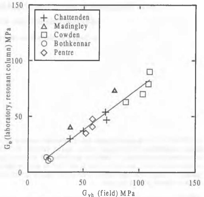
Figure 2: Comparison of stiffness from field shear wave measurements and laboratory resonant column tests.
