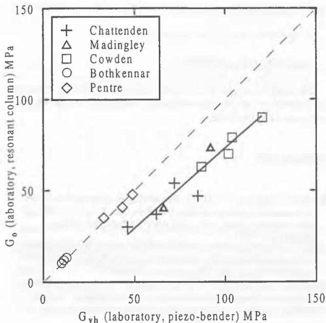
Figure 3: Comparison of G from laboratory tests
