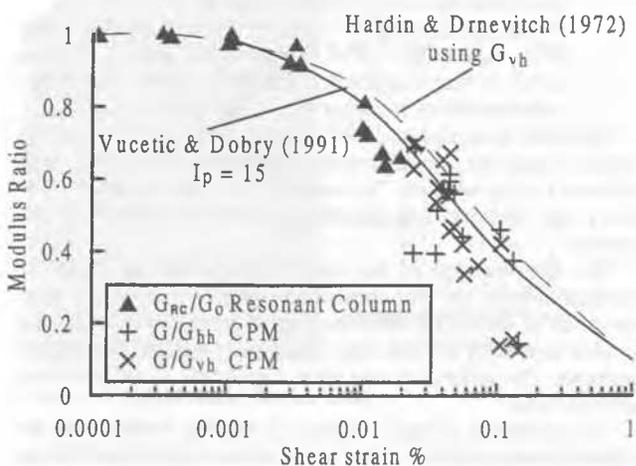
Figure 5: Resonant column and CPM data from Pentre site
