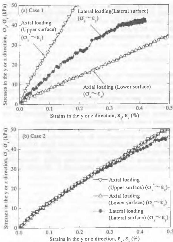
Figure 3. Stress-strain relationships on the dummy specimen.
