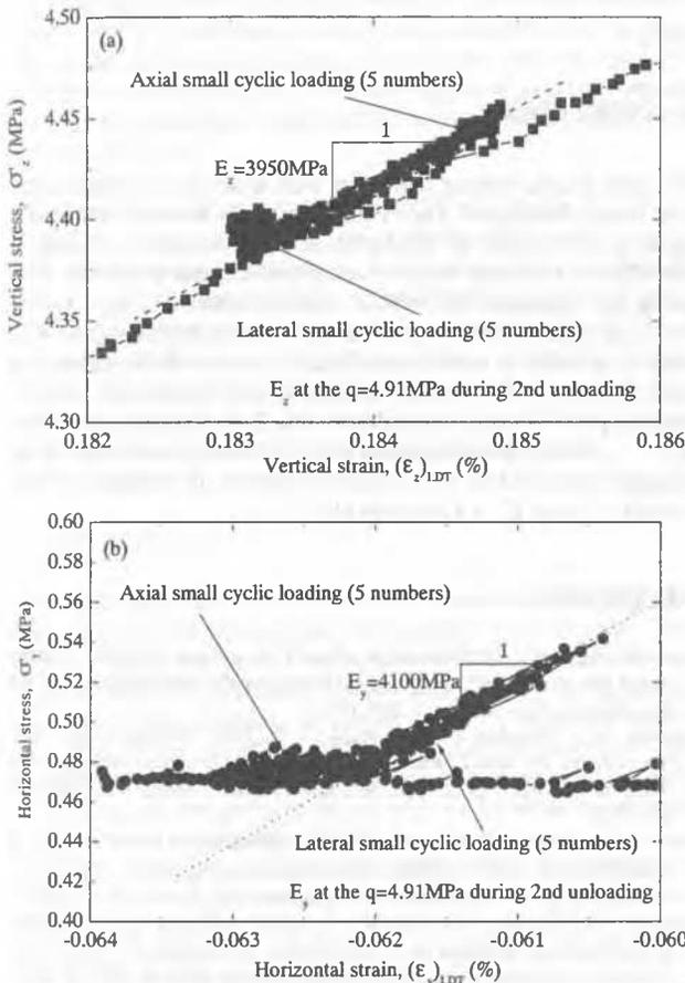
Figure 6. Stress-strain relationships from typical cyclic tests.
