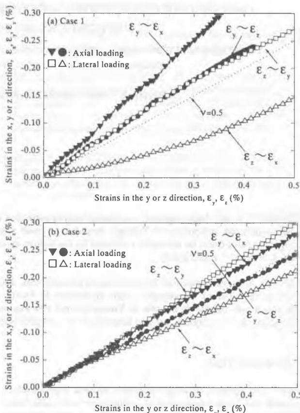
Figure 4. Strain-strain relationships on the dummy specimen.
