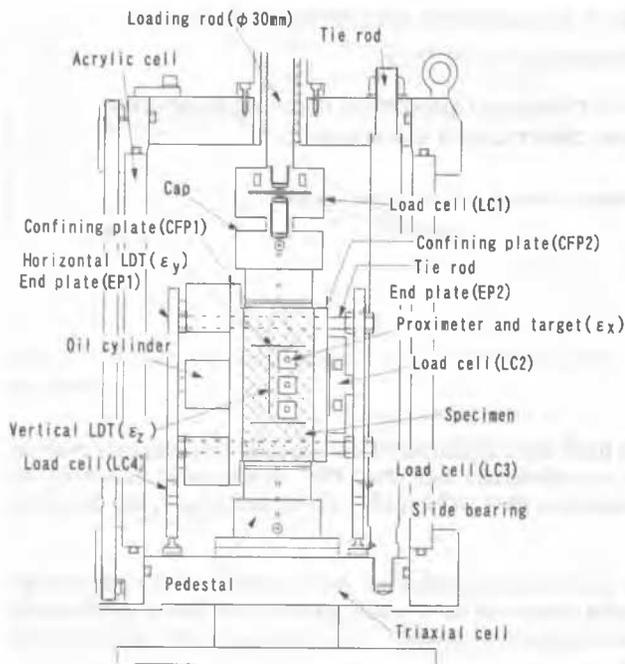
Figure 2. Triaxial cell with lateral loading system.
