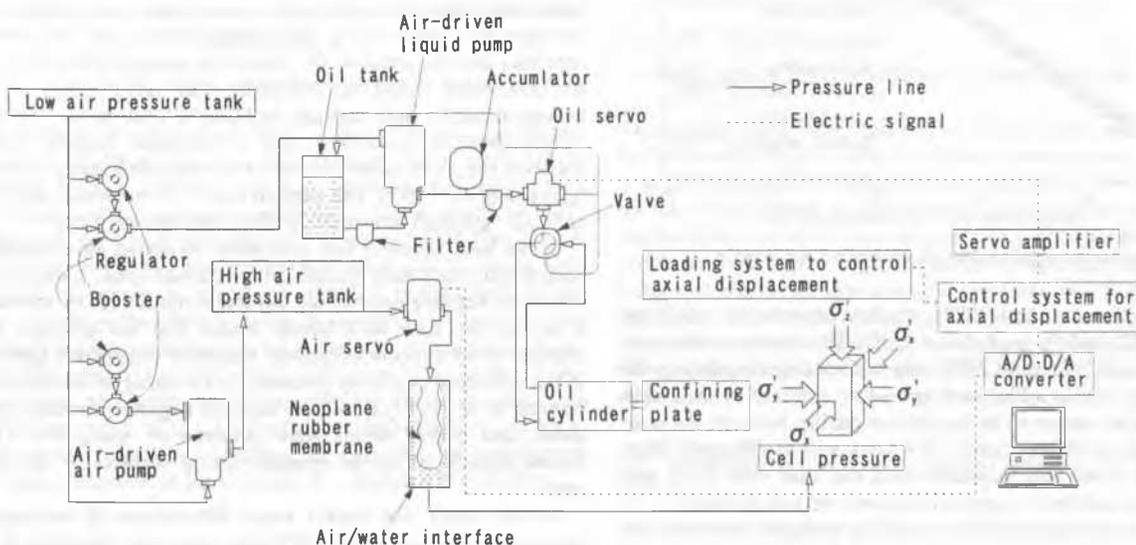
Figure 1. True triaxial testing system.
