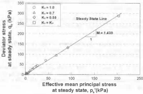
Figure 5. Unique relationship between deviator stress and effective mean principal stress at steady state
