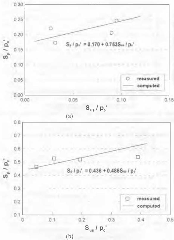
Figure 10. Comparison of the computed and measured values for  $S_p/p'_c$  -  $S_{us}/p'_c$  relation
