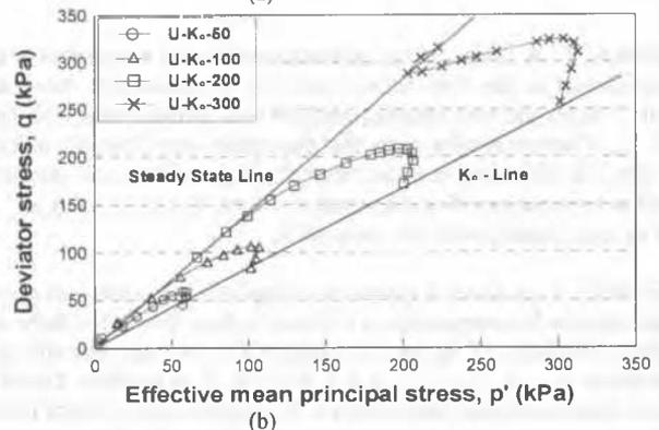
Figure 3. Undrained behavior for anisotropic consolidation ( $K_c = K_o$ )
