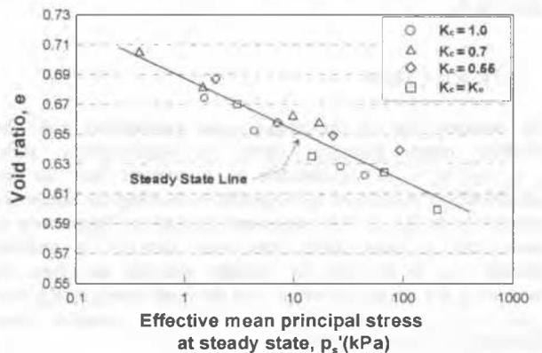
Figure 4. Relationship between void ratio and effective mean principal stress at steady state
