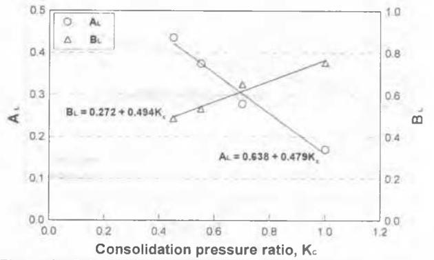
Figure 9. Relationship between consolidation pressure ratio and parameters  $A_L$  and  $B_L$
