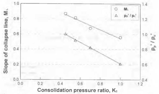
Figure 8. Variation of the slope of collapse line  $M_L$  and  $p_p'/p_c'$  with different consolidation pressure ratio
