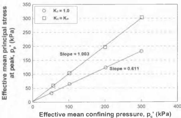
Figure 7.  $p_p' - p_c'$  relationship for isotropic and anisotropic consolidations
