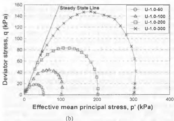
Figure 2. Undrained behavior for isotropic consolidation
