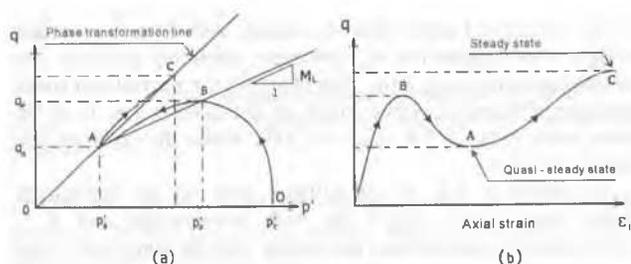
Figure 1. Characteristics of undrained behavior of loose sand (Ishihara, 1993)
