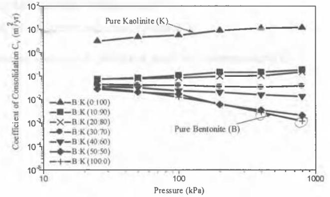
Figure 2: Coefficient of consolidation  $C_v$  vs pressure for bentonite-kaolinite (B:K) mixes
