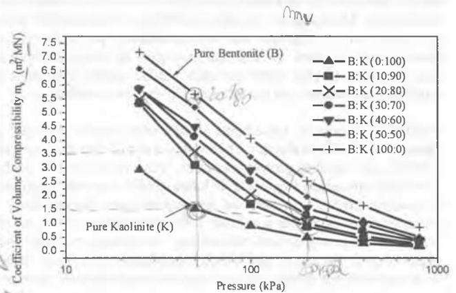
Figure 3: Coefficient of volume compressibility  $m_v$  of bentonite-kaolinite (B:K) mixes
