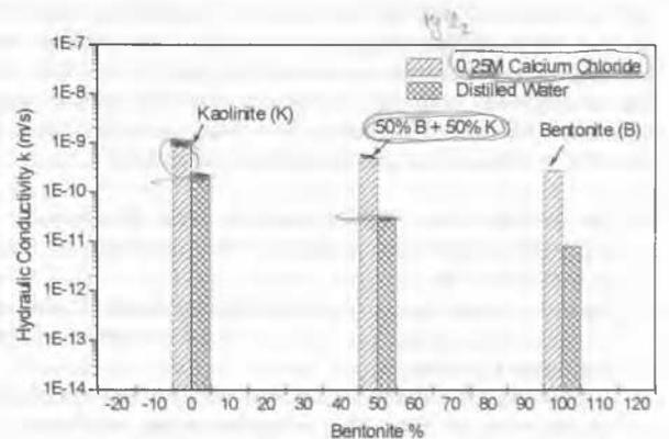
Figure 9. Variation of hydraulic conductivity *k* (m/s) in B:K mixes using falling head method. (Permeant: distilled water and 0.25M CaCl<sub>2</sub>, Consolidation pressure: 35 kPa)
