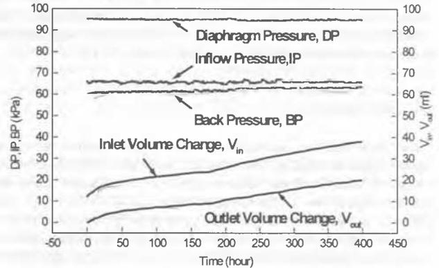
Figure 7. Determination of hydraulic conductivity *k* (m/s) with the constant head method in Rowe cell (Permeant: distilled water, Consolidation pressure: 35 kPa, B:K=50:50 mix)
