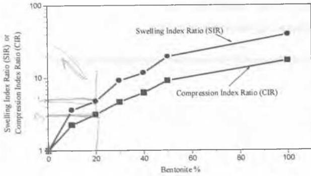
Figure 1. Variation of swelling index ratio (SIR) and compression index ratio (CIR) with bentonite percentage
