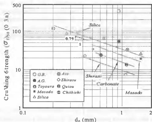
Figure 4. Dependency of  $(\sigma_f)_{50}$  on  $d_0$ .
