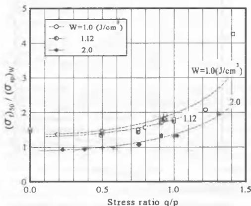
Figure 10. Ratio  $(\sigma_l)_{50}/(\sigma_{sp})_W$  plotted against to stress ratio.
