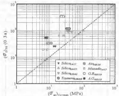
Figure 7.  $(\sigma_f)_{50}$  plotted against  $(\sigma_{sp})_{Cc=max}$ .
