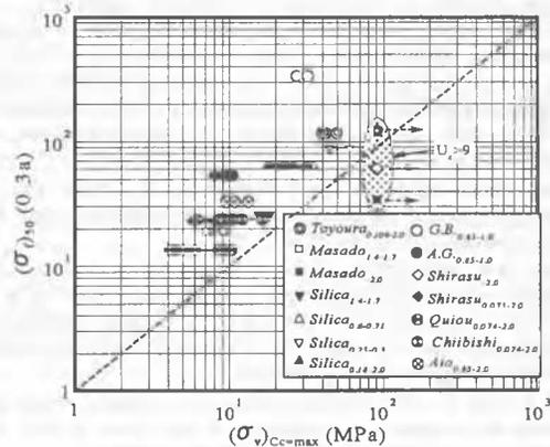
Figure 6. Relationship between  $(\sigma_f)_{50}$  and  $(\sigma_v)_{Cc=max}$ .
