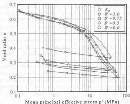
Figure 9.  $e - \log p$  curves for Silica<sub>1.4-1.7</sub> subjected to stress ratio ( $q/p$ ) constant and  $K_0$  compression.
