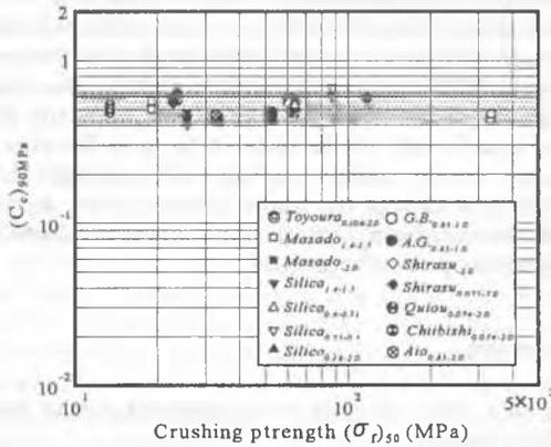
Figure 5.  $(C_c)_{90MPa}$  related to  $(\sigma_f)_{50}$ .
