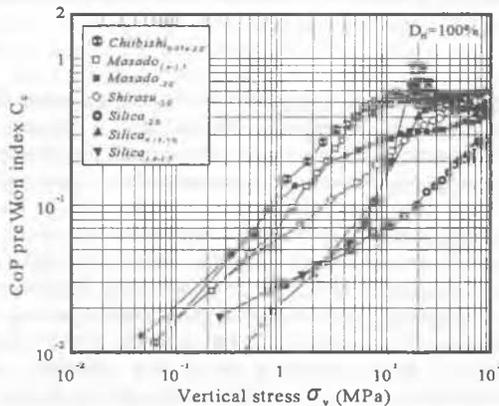
Figure 2. Variation of compression index as vertical stress increase.
