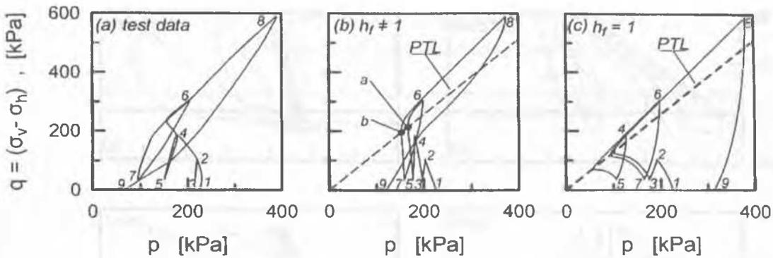
Figure 1. Comparison of test data to simulations of an undrained triaxial path including shear reversals: a) test data (from Ishihara et al. 1975), b) simulation, which accounts for fabric evolution ( $h_f \neq 1$ ), c) simulation, which ignores fabric evolution ( $h_f = 1$ ).
