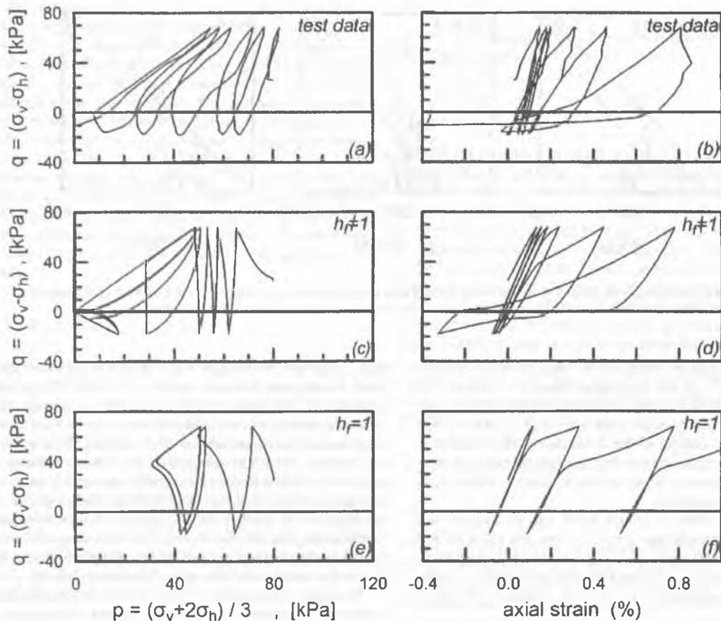
Figure 2. Comparison of test data to simulations of an undrained cyclic triaxial test: a & b) test data (from Arulmoli et al. 1992), c & d) simulation, which accounts for fabric evolution ( $h_f \neq 1$ ), e & f) simulation, which ignores fabric evolution ( $h_f = 1$ ).
