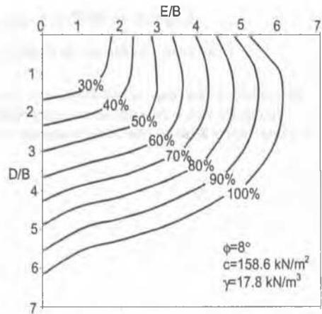
Fig.2 Contours of Equal Percentage of No-Void Ultimate Bearing Capacity for W/B=3.0
