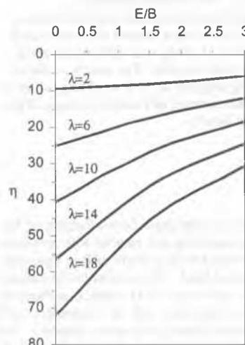
Fig.3 (A) Contours of 100% No-Void Ultimate Bearing Capacity
