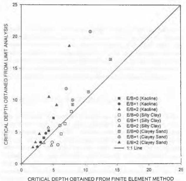
Fig.5 Comparison of Critical Depth Obtained from Limit Analysis and Finite Element Method
