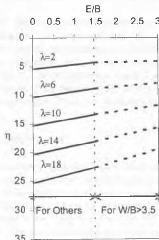
Fig.3(C) Contours of 50% No-Void Ultimate Bearing Capacity
