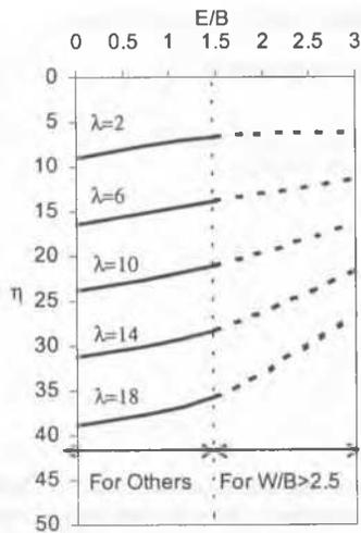
Fig.3(B) Contours of 75% No-Void Ultimate Bearing Capacity
