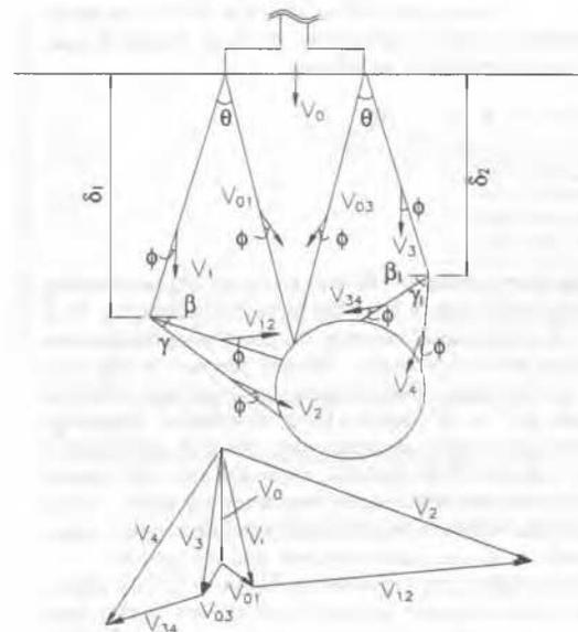
Fig.1 Failure Mechanism and Hodographs
