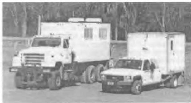
Figure 2. Louisiana cone penetration systems: REVEGITS cone truck on the left and CIMCPT cone truck on the right.
