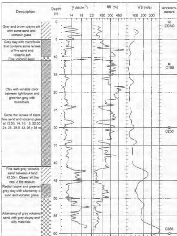
Figure 2. Profiles of stratigraphy, unit weight,  $\gamma$ , water content,  $w$ , shear wave velocity,  $V_s$ , and location of accelerometers at CAO site.
