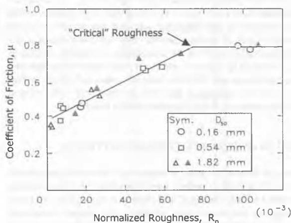
Figure 1. Relationship Between Surface Roughness and Interface Friction (after Uesugi and Kishida, 1986).
