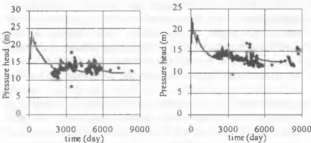
Figure 4 The measured and computed pressure head underneath B22 section at BH-1(-12.50 m).
