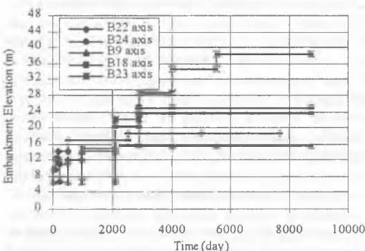
Figure 2. The staged construction program of the dam.
