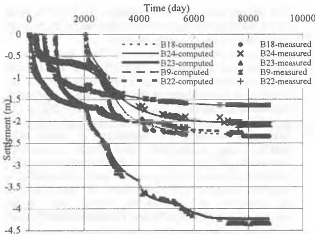
Figure 3 Computed and measured settlements in section of B22, B18, B23, B24 and B9.
