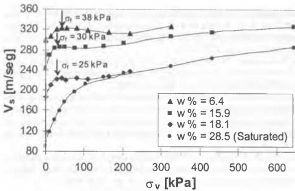
Figure 5: Small-strain response. Variation of shear wave velocity with vertical pressure for undisturbed specimens of unsaturated loess (data from Clariá and Rinaldi, 2000).
