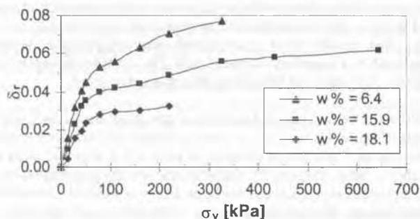
Figure 4: Variation of the coefficient of collapsibility with pressure for the undisturbed and unsaturated specimens (refer to Figure 3).
