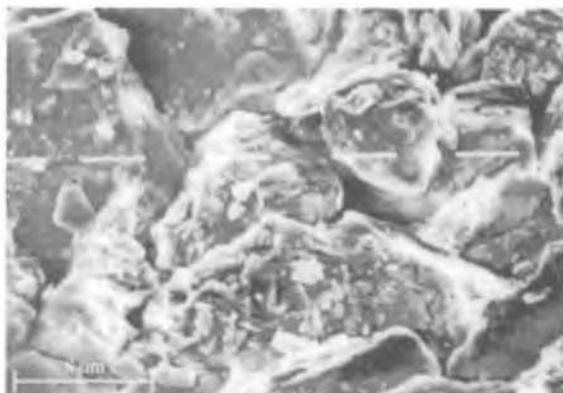
Figure 1.b: SEM photograph (X250) of sand and silt particles of loess.
