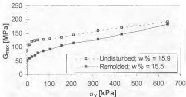
Figure 9: Shear modulus measured for unsaturated remolded and undisturbed specimens of loess. Specimens have similar moisture content and dry unit weight.
