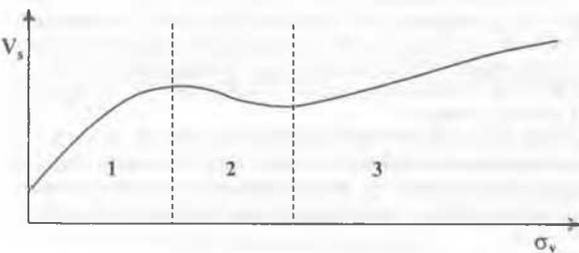
Figure 6: Velocity-stress response of unsaturated, undisturbed loess. 1: Low stress range: hairline cracks close and early local collapse develops; strain energy is stored. 2: Massive collapse of the structure and closure of macropores. 3: Re-structuring. The effect of the state of stress exceeds the effect of suction and any remaining bonding.
