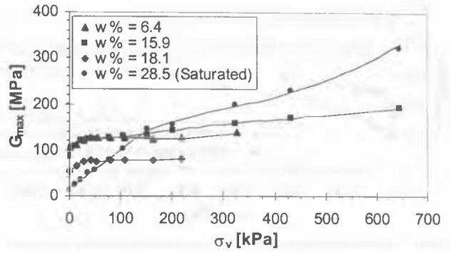
Figure 7: Variation of shear modulus  $G_{max}$  with vertical pressure for undisturbed specimens of loess.
