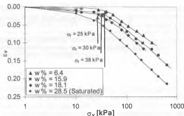
Figure 3: Load-deformation response of undisturbed specimens of loess subjected to  $k_c$  loading (modified from Clariá and Rinaldi, 2000).
