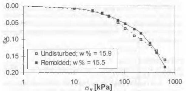
Figure 8: Compressibility curves for remolded and undisturbed loess at similar moisture content and dry unit weight.
