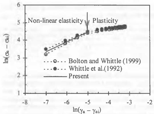
Figure 2. Deriving the power law relationship from a reloading loop
