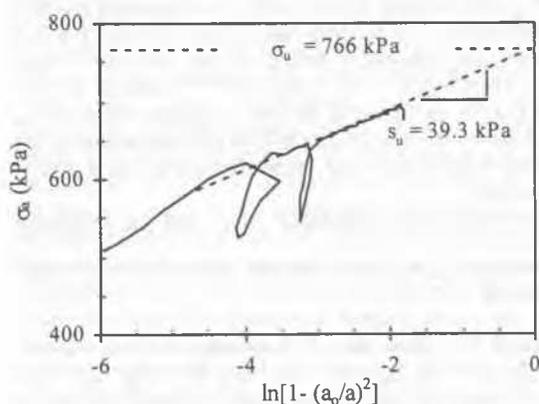
Figure 4. Determination of undrained shear strength and ultimate pressure from the pressuremeter expansion curve
