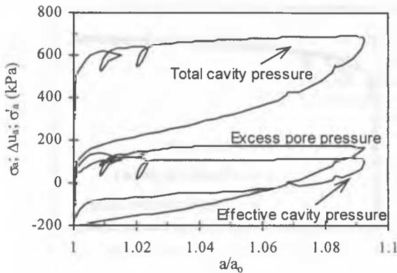
Figure 1. A typical self-boring pressure test results in the Singapore marine clay
