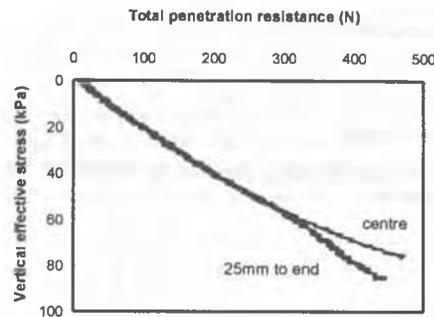
Figure 5. Penetration resistances after the earthquake saturated sand model.
