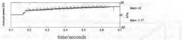
Figure 7. Long term excess pore pressure-time history of PPT6671 on the bottom of the container.
