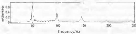
Figure 8. Fourier analysis of the input acceleration signal for *c1*.
