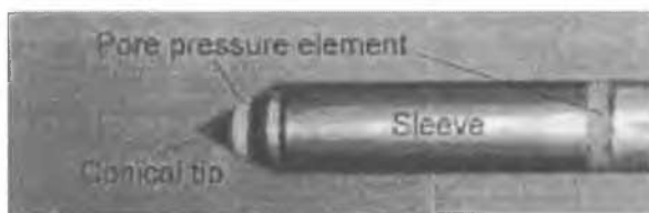
Figure 1. Picture of the piezocone penetrometer with dual pore pressure elements u_1 at the cone tip and u_2 behind the sleeve.
