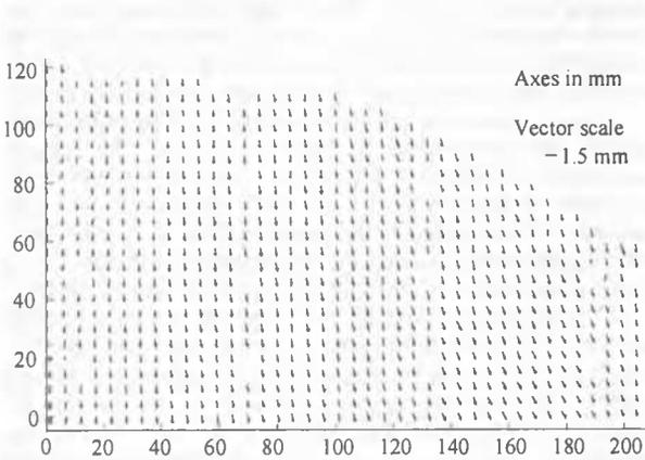
Figure 8. Displacement vectors following camera calibration
