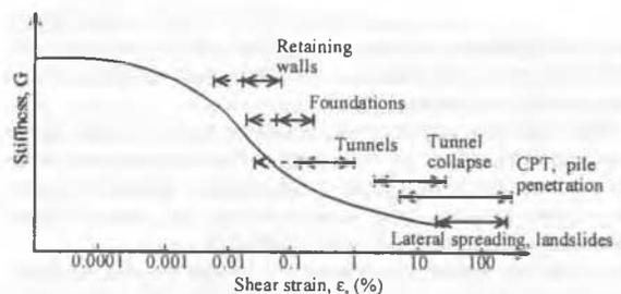
Figure 1. Typical strain ranges in geotechnics (after Mair, 1993)
