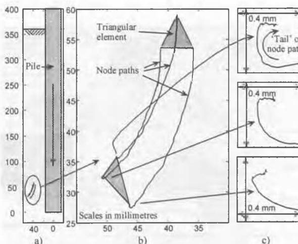
Figure 5. Selected node paths during pile penetration
