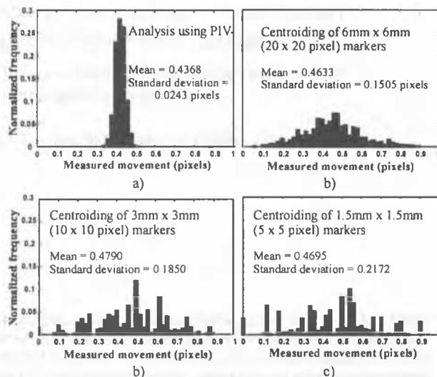
Figure 2. Comparative precision of PIV and centroiding methods
