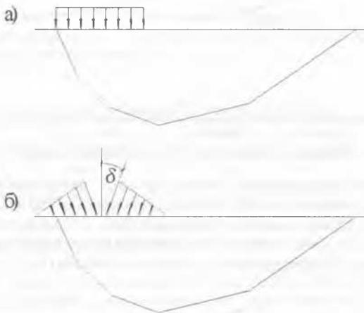
Figure 3. Diagram used to calculate bearing capacity of cohesive (a) and cohesionless (b) beds.
