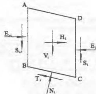
Figure 2. General diagram of forces acting on slice.
