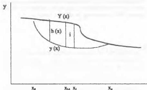
Figure 1. Schematic diagram used for slope stability analysis
