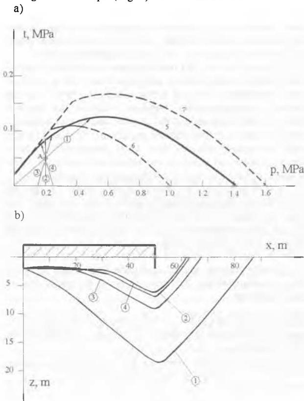
Figure 4. Foundation stability envelope (a) and failure lines (b): 1-4 – loading paths and respective failure lines; envelopes: 5 – MVLm; 6 – Brinch Hansen (1970); 7 – Caquot & Kerisel (1953)
