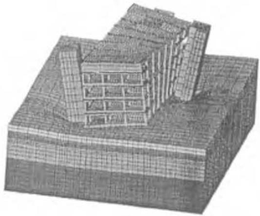
Figure 2. Deformations of the building as shown by the calculations (deformation scale enlarged by 50)
