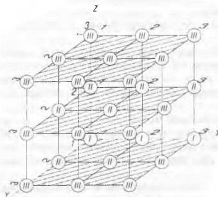
Figure 1. Identification of geotechnical complexity of new construction or reconstruction in city areas: *x* - technical *condition* of adjacent structures; *y* - *risk*, *z* - *importance* of new construction or reconstruction.
