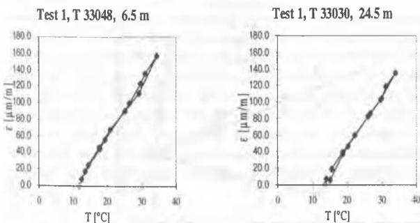
Figure 5. Evolution of strains during thermal solicitation at depths 6.5 and 24.5 m -Test 1
