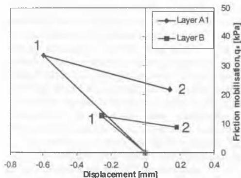
Figure 13 : Mobilisation of side friction by building weight (1) and thermal solicitation (2)
