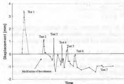
Figure 7. Vertical displacement of the pile head
