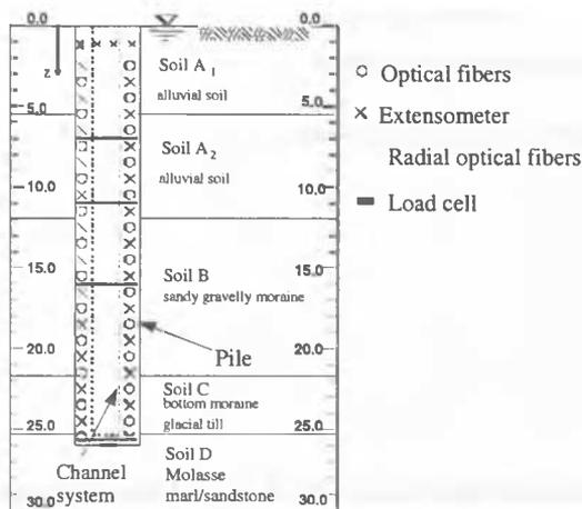
Figure 2. Stratigraphic profile and instrumentation of the test pile
