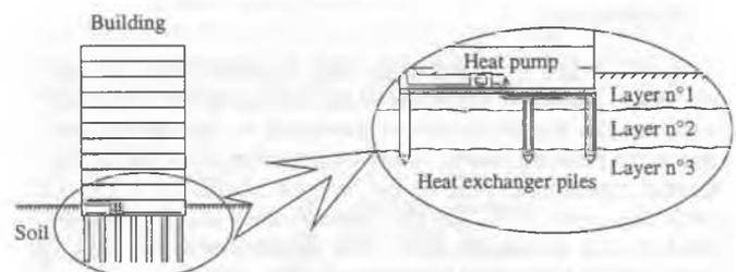
Figure 1. Schematic representation of a heating system with heat exchanger piles
