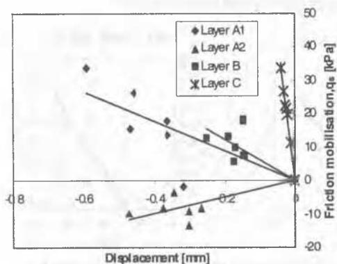
Figure 11. Side friction mobilised by the building weight.
