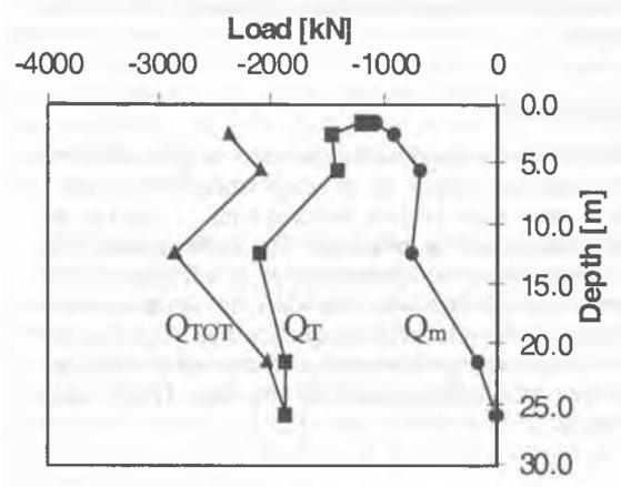
Figure 10. Mechanical ( $Q_m$ ), thermal ( $Q_T$ ) and total ( $Q_{TOT}$ ) loads in the pile after building construction
