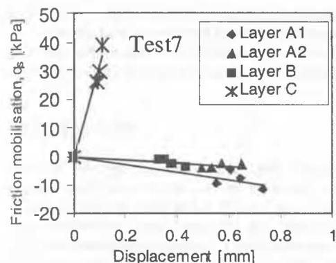
Figure 12. Side friction mobilised by the thermal solicitation (a) Test1; (b) Test7
