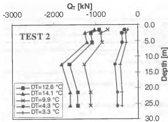
Figure 8. Load evolution during the thermal cycle – Tests 2 and 6
