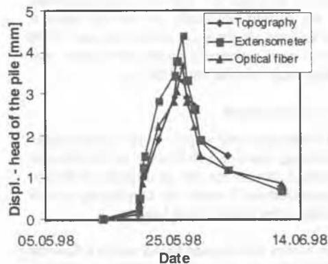
Figure 6. Pile displacement during Test 1
