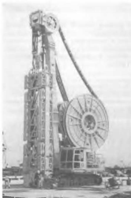
Figure 2. Diaphragm walling cutter BC 40
