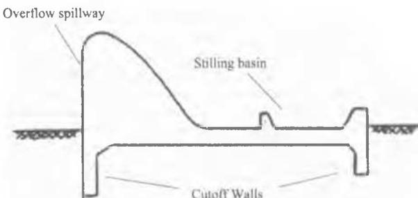
Figure 1 A typical cross section for the diversion dams.
