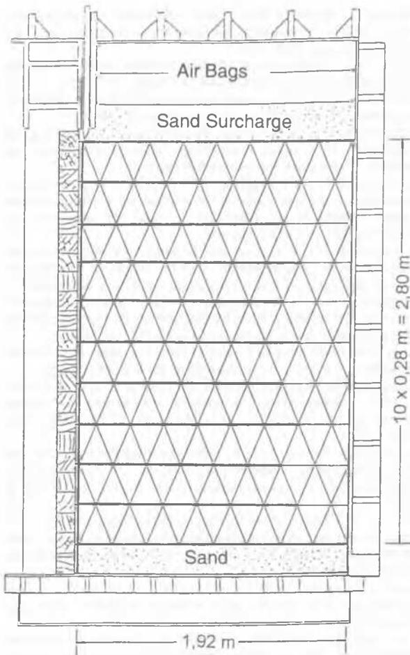
Figure 2. Denver wall (mesh A).
