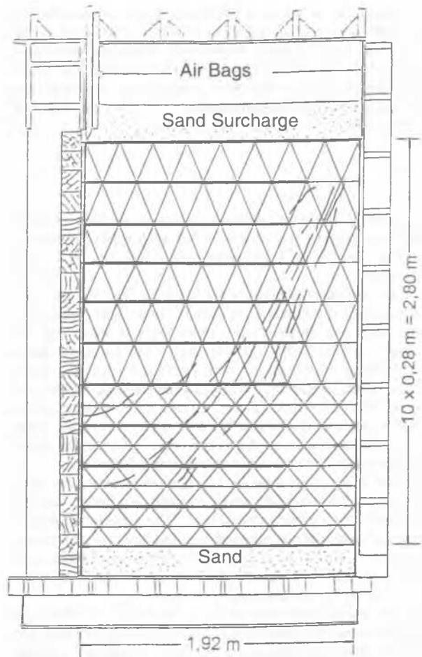
Figure 3. Denver wall (mesh B) and observed slip lines.
