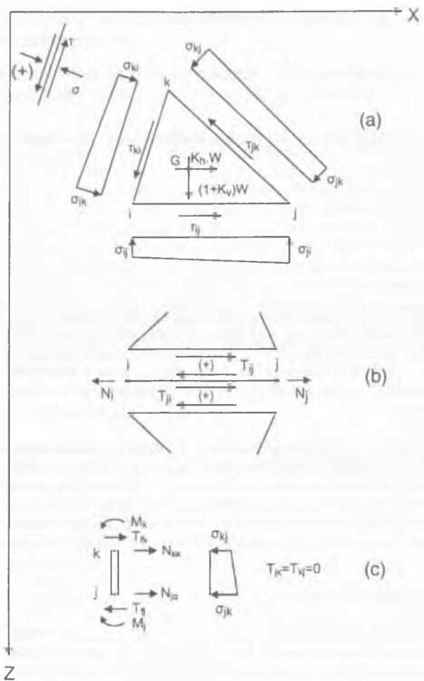
Figure 1. Free body diagrams for three typical elements.
