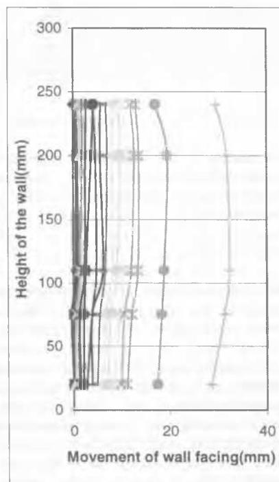
**Figure 7 – Outward Movement of the Wall Facing Loading Behind the Anchor Zone**
