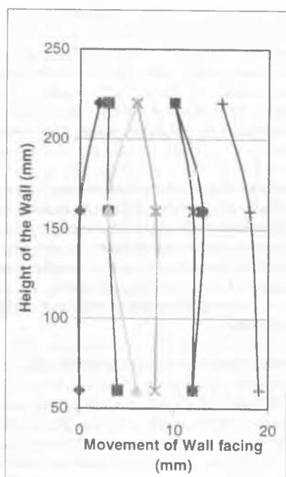
**Figure 6 – Outward Movement of the Wall Facing with Loading within the anchor zone**
