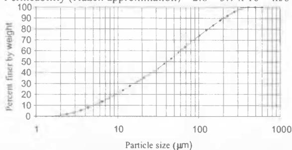
Figure 2. Grain size distribution for BHP Cannington tailings
