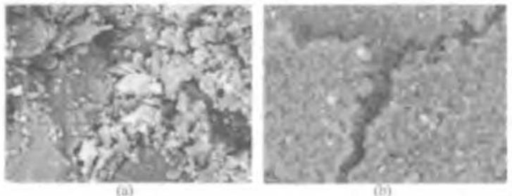
Figure 1. Scanning electron microscope images (a) tailings only (b) paste fill mix (4% cement, 76% solids)
