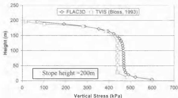
Figure 6. Vertical stress profile down the center of the primary stope
