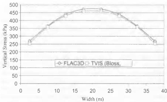
Figure 7. Vertical stress profile across the center of the primary stope.
