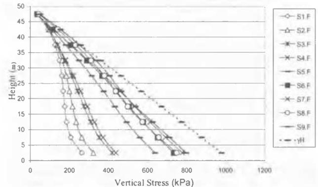
Figure 9 Vertical stress profile down the center of the primary stope, during the filling sequence.  $\gamma H$  = ore unit weight \* height – used as a comparative value to assess the extent of support provided by arching.
