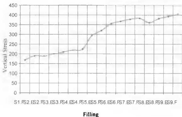
Figure 8. Vertical stress measured in the center of the primary stope (stope 1) at a height of 25m during the mining sequence. S1F = Stope 1 Filled, S2.E = Stope 2 Excavated.
