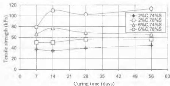
Figure 3. Progressive tensile strength results
