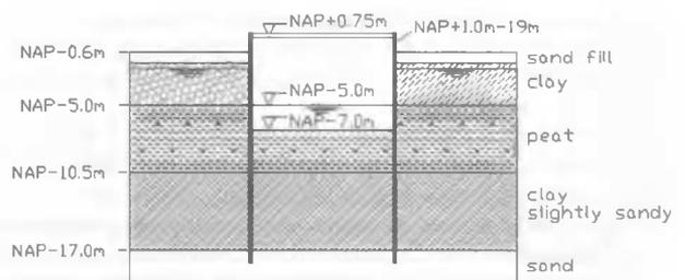
Figure 2. Side view of the Rotterdam sheet pile wall field test.
