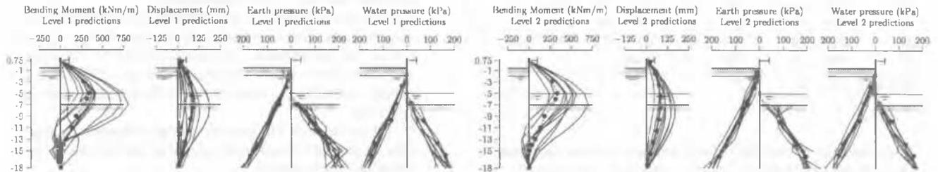
Figure 4. Level 1 and level 2 predictions for the Larssen 607K-wall in construction stage III. The bullets indicate the measured results.
