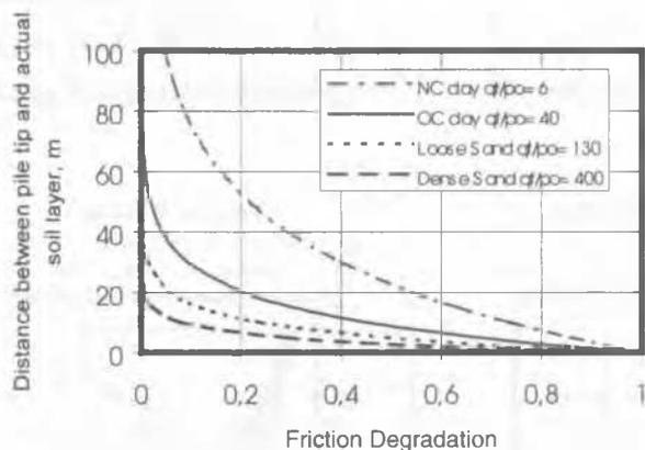
Figure 2. Examples of degradation shapes for different soils
