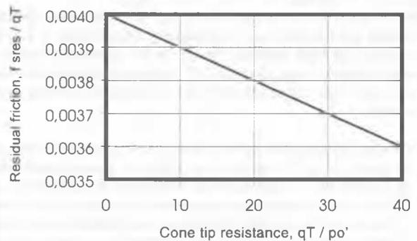
Figure 1. Residual clay friction ratio vs. cone resistance ratio
