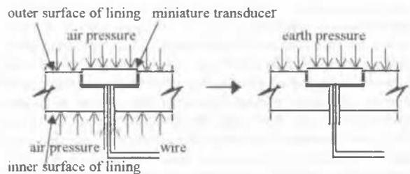
(a) air support pressure acting (b) earth pressure acting without air pressure
