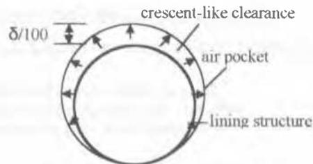
Figure 3. Scheme of model clearance
