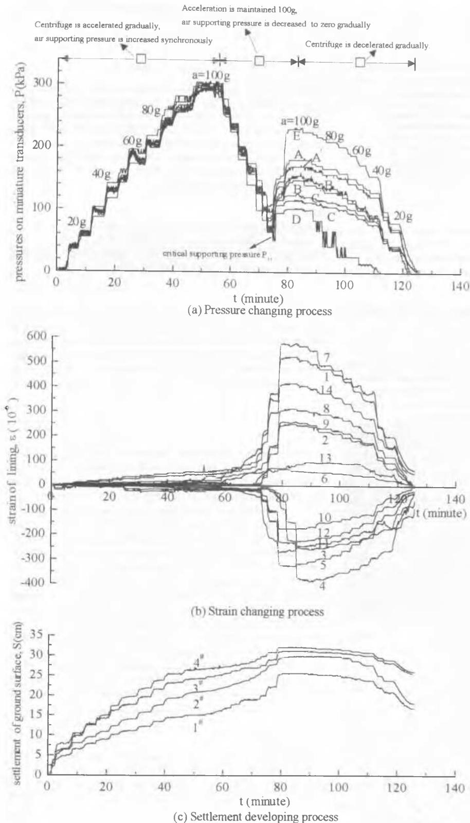
Figure 4. Pressure, strain and settlement measured in centrifuge accelerating and decelerating processes ( $H/D=2$ , dry sand ground,  $\delta=100\text{mm}$ )
