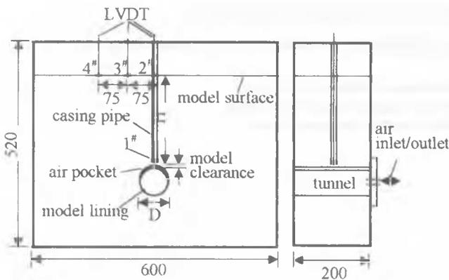
Figure 1. Sketch of 2-D model and its container, in mm
