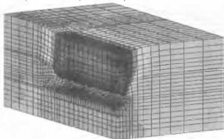
Figure 7 3-dimensional finite element analysis of surface settlements with the groutpressure model
