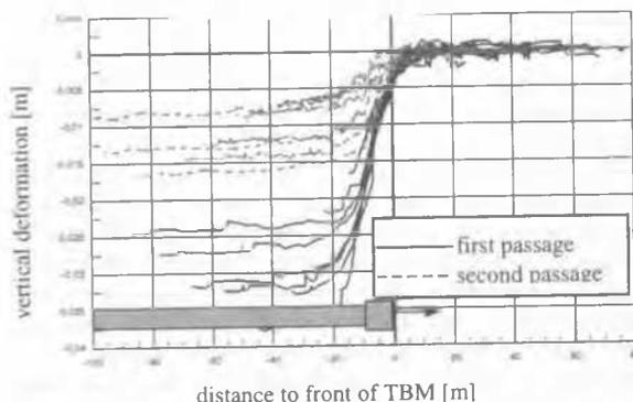
Figure 3 Green field settlements above tunnel axis at Northern Monitoring Area
