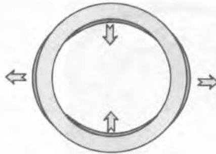
Figure 16. Differential deformations due to ovalisation
