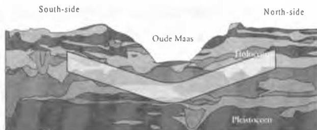
Figure 4. Geotechnical Profile at the 2nd Heinenoord Tunnel
