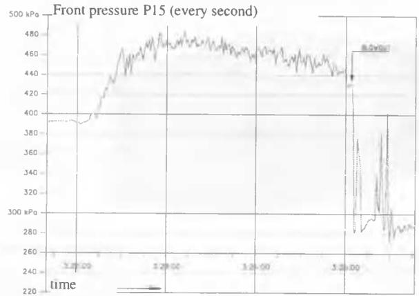
Figure 13. bore front pressure at time of the blowout
