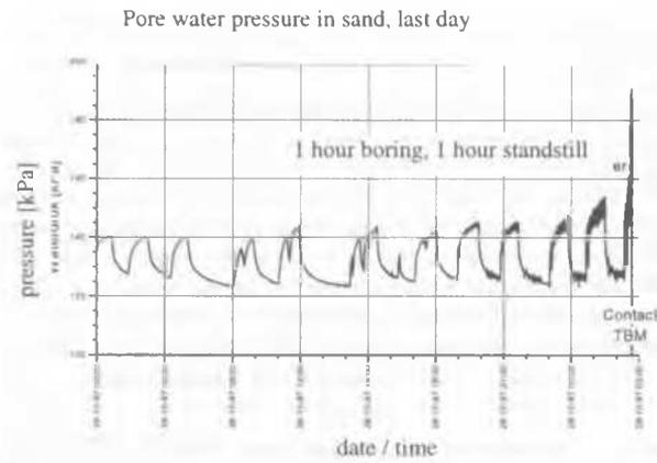
Figure 9. pore-water pressure in sand layer last day
