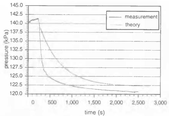
Figure 8. Pore pressure measurements as a function of time after stopping of the excavation of the TBM, 1.8 m from the measuring device
