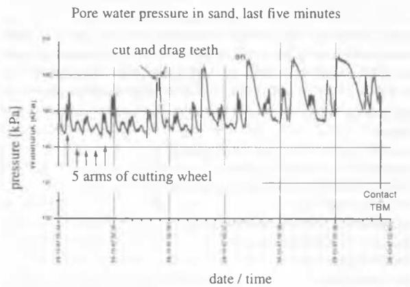
Figure 10. pore-water pressure in sand last minutes
