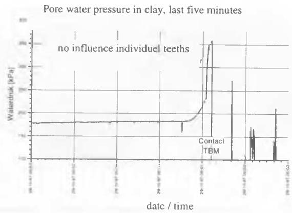
Figure 12. pore-water pressure in clay last minutes
