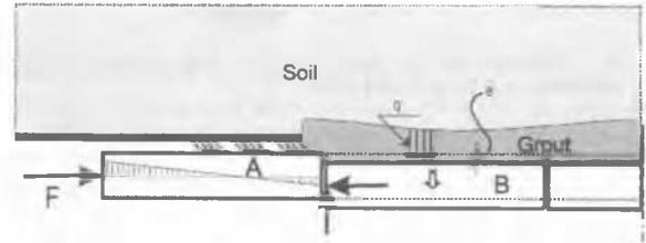
Figure 17. Eccentricities due to partial loading during tunnel construction of the tunnel lining, where tunneling a is unloaded in radial direction and tunneling b is subjected to radial loads by grouting-pressures
