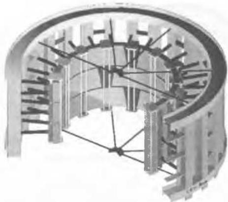
Figure 18. Experimental test setup for large scale testing of tunnel loading situations, (v.d Horst et al 1999)
