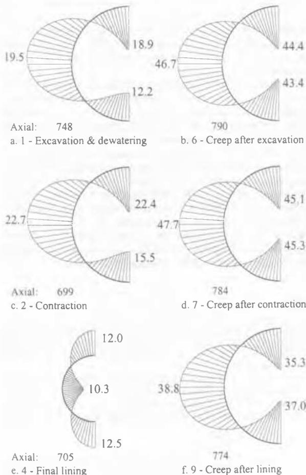
Figure 2. Overview of bending moments from different calculation phases (values in kNm/m). Indication of axial forces in kN/m.
