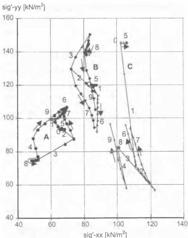
Figure 3. Effective stress paths of points A (above), B (left) and C (below the tunnel). The numbers refer to the calculation phases. The arrows indicate the stress development during the creep phases.
