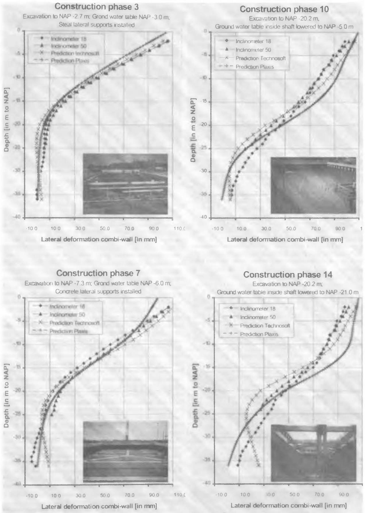
Figure 4. Measured versus predicted lateral deformations.
