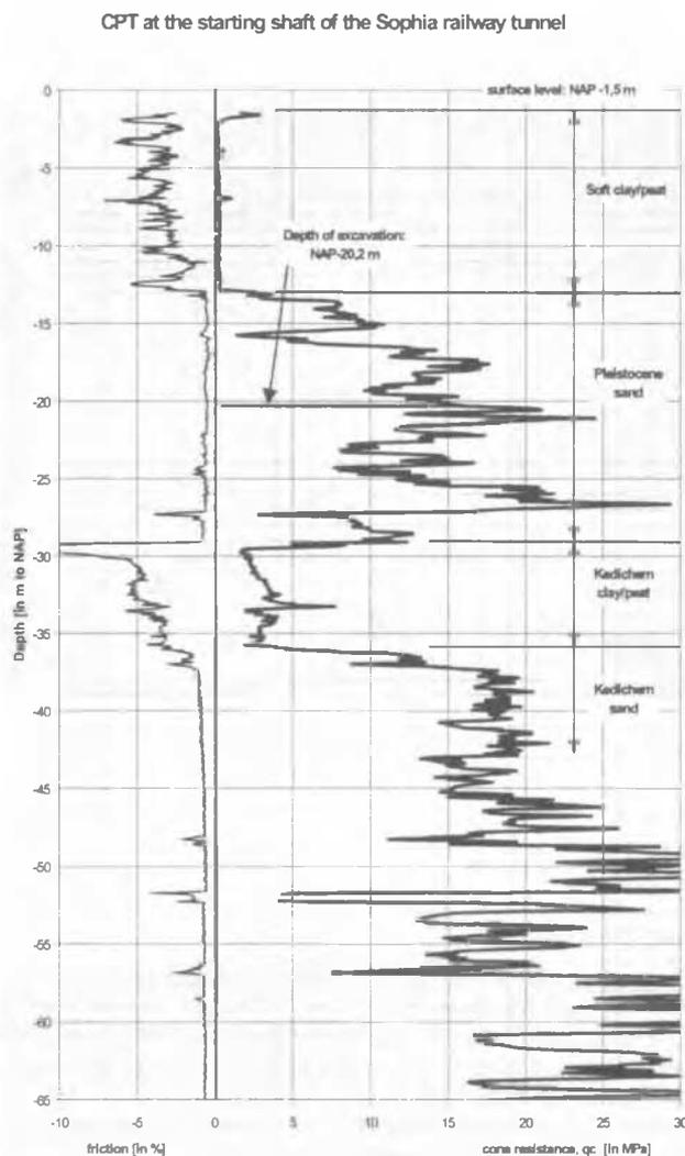
Figure 2. CPT and soil profile at the starting shaft.
