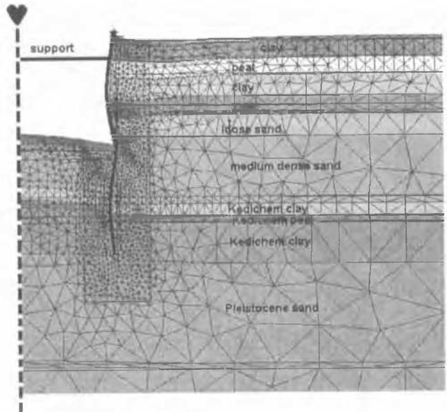
Figure 6. Calculated deformations starting shaft., FEM analysis
