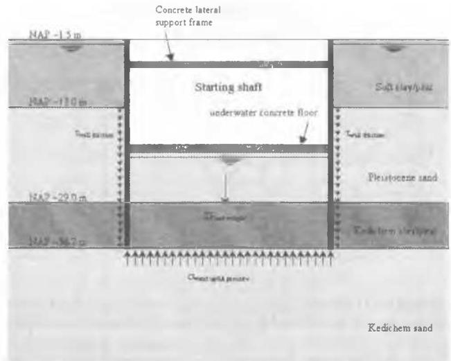
Figure 3. Vertical equilibrium of the starting shaft in construction phase 14 (excavated and dewatered).
