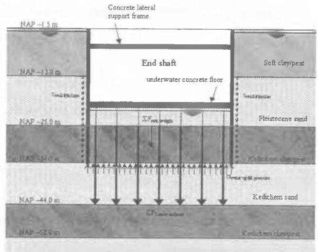
Figure 8. Vertical equilibrium of the end shaft in the final phase.
