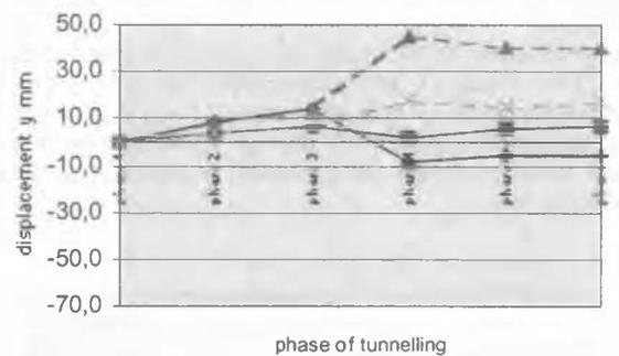
Figure 8. Vertical displacement versus phase of tunnelling Point C
