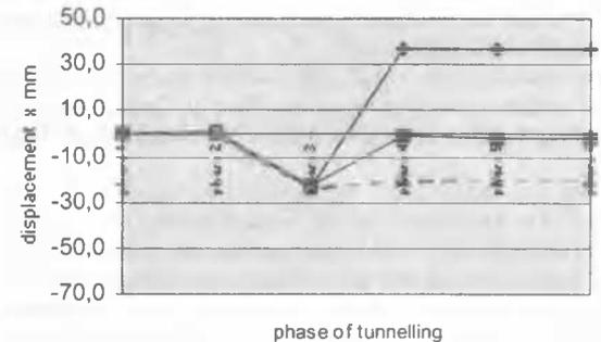
Figure 7. Horizontal displacement versus phase of tunnelling Point C
