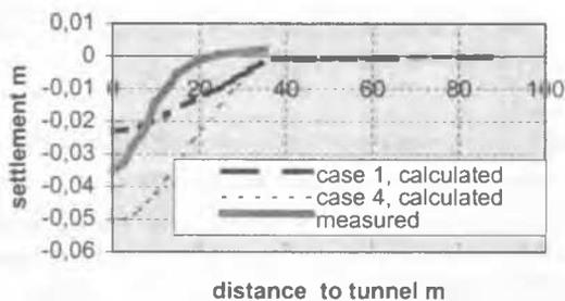
Figure 10. Predictions (HS model) and measured data after boring.
