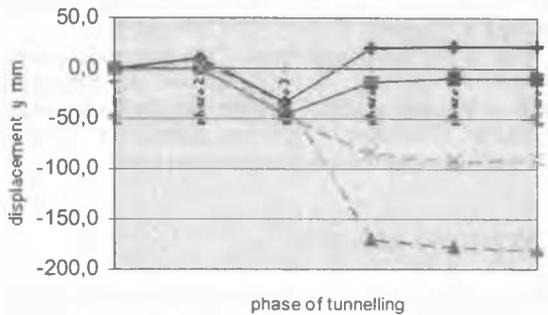
Figure 4. Vertical displacements versus phase of tunnelling Point B.
