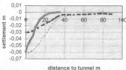
Figure 11. Predictions (HS model) and measured data after consolidation.
