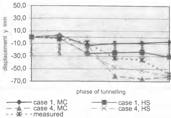
Figure 3. Vertical displacement versus phase of tunnelling Point A.
