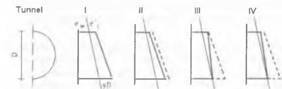
Figure 2. Grouting pressure distribution along lining.
