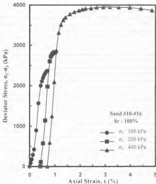
Figure 3. Stress – strain curves from M-UU triaxial compression test.
