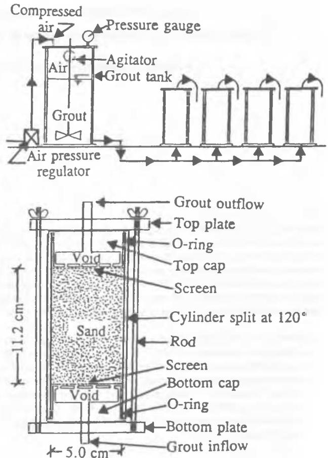
Figure 2. Apparatus for grouting sand specimens.
