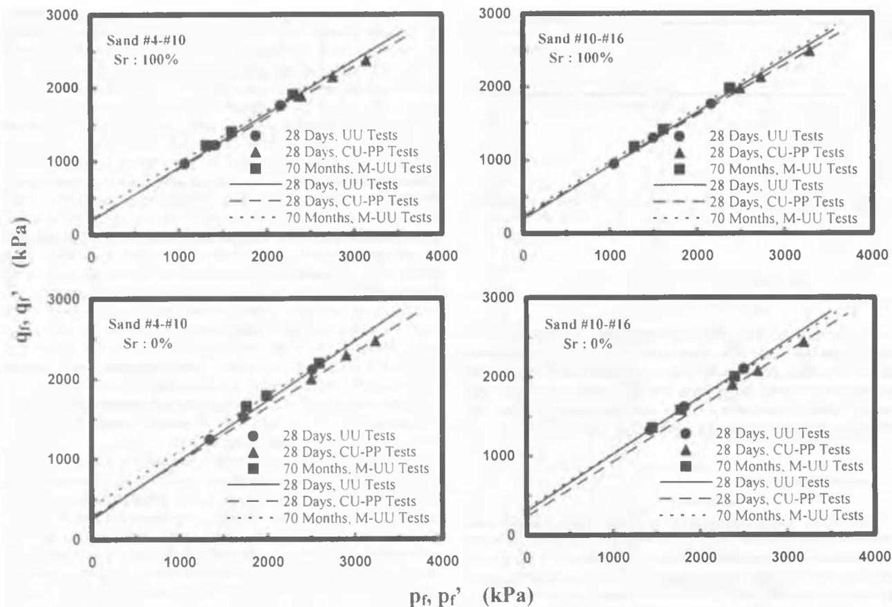
Figure 4 Failure envelopes for PFA grouted sands from triaxial compression tests.
