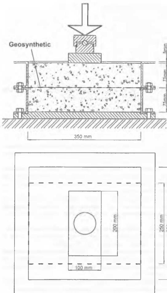
Figure 3. Scheme of the laboratory test apparatus (ENV ISO 10722-1). Top: cross section view, below: plan view.
