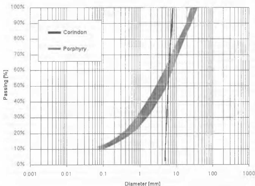
Figure 1. Grain size distribution of the two soils used in the damage installation tests
