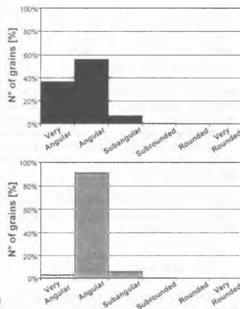
Figure 2. Angularity of the grains of the two soils used in the damage installation tests
