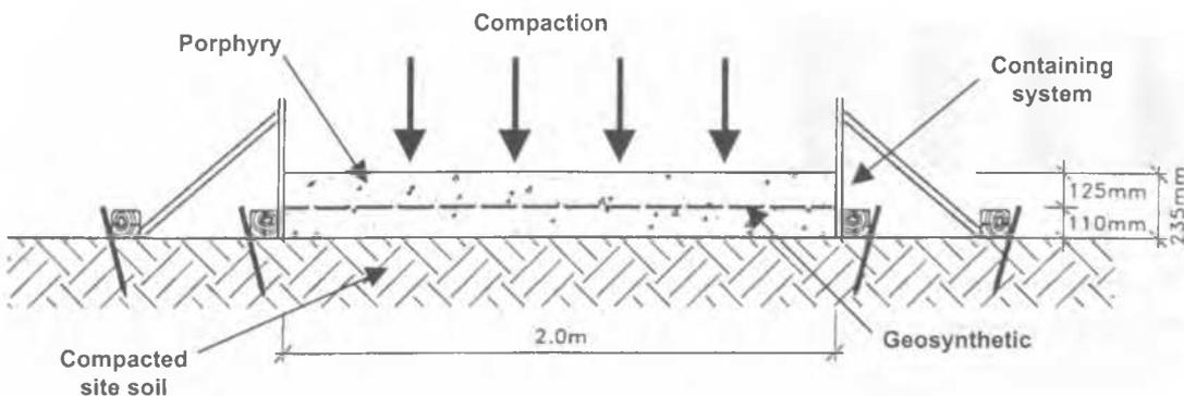
Figure 4. Cross section of the full scale field test
