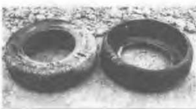
Figure 2. Full tire and sidewall removed tire.
