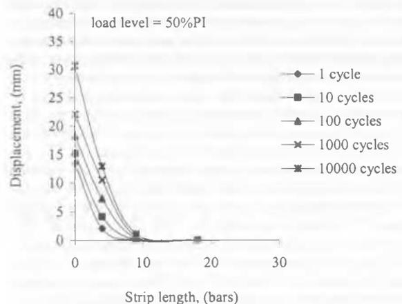
Figure 5. Strain variation due to cyclic loading.
