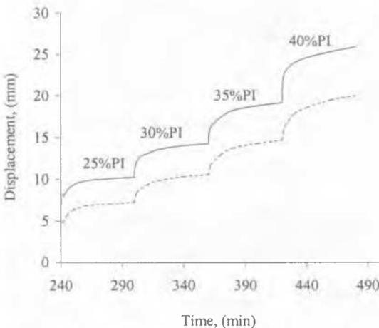
Figure 6. Total deformation-time relationships with applied load.
