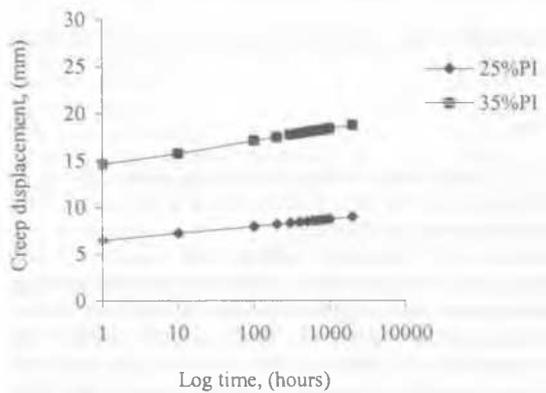
Figure 10. Long-term creep displacement-time relationships.
