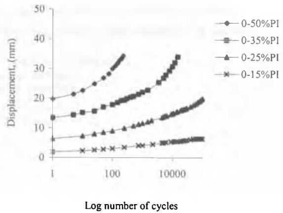
Figure 3. Load-displacement relationships due to cyclic loading.
