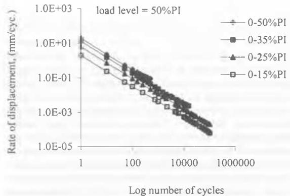
Figure 4. Rate of displacement-load cycles relationships.
