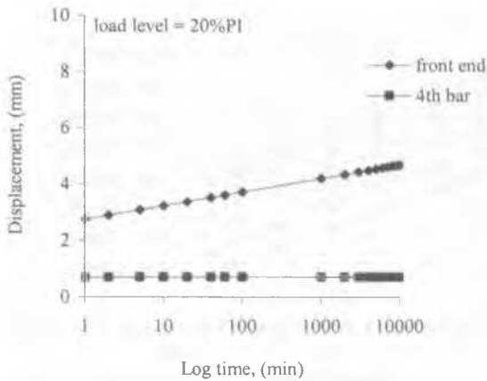
Figure 9. Creep displacement-log time relationships at various sections.
