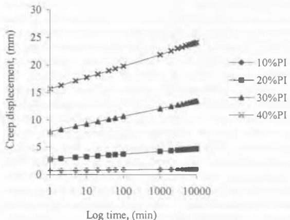
Figure 8. Medium-term creep displacement-log time relationships.
