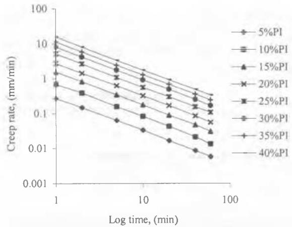
Figure 7. Creep deformation rate-time relationships.
