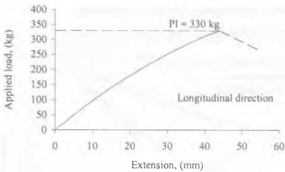
Figure 2. SR2 geogrid tensile strength extension relationship.
