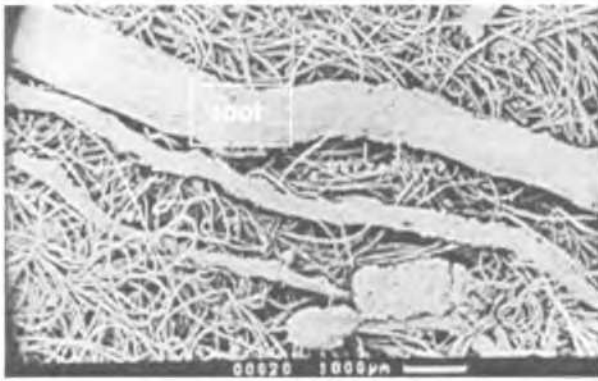
Figure 9. Roots in top filter (SEM)
